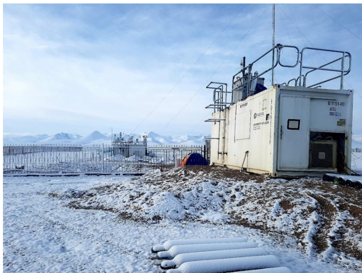
The Leeds FAGE instrument for the measurement of radicals at 4730 m in Tibet
