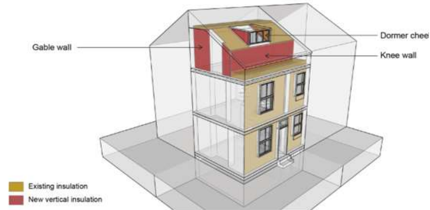
Figure 1-7 Stage 2: Roof retrofit to Bedroom 2 (17BG.A.R)
